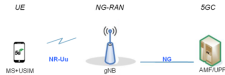
Figure 1: Showcases a simplified diagram of how user equipment connects to cellular towers and the core network. [1]
